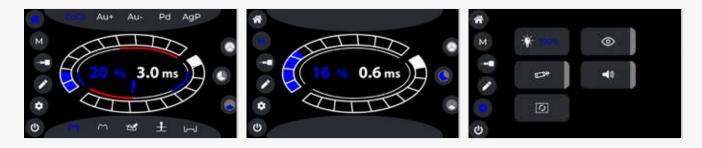
Optimised settings menu with practical additional functions such as the enhanced micro mode, the retention welding mode, or the fixation welding function. Basic functions are selected in just a few steps in the settings menu.
