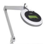
LCD eye protection system consisting of LED magnifier luminaire with lighting 7.5 W, magnification 2.25x (5 dpt) and electronically controlled eye-protecting filter (luminescence DIN3 / obscurity DIN11).
