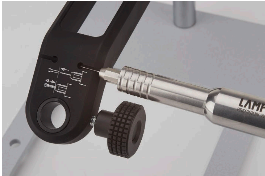
Fig. 5.2 Adjusting electrode length with handpiece holding arm
