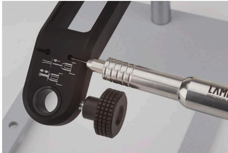
Fig. 5.2 Adjusting electrode length with handpiece holding arm
