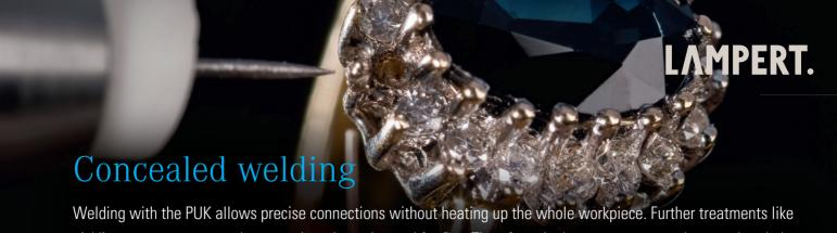
Welding with the PUK allows precise connections without heating up the whole workpiece. Further treatments like pickling are not necessary because there is no demand for flux. Therefore single components can be completed already before assembling. Surfaces can be finished or for example enamelled or lacquered in advance. Of course, already set stones are no problem as well.
