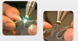
In order to strengthen the point of breakage, we recommend our Pd/Ag welding wire that you can obtain from your PUK dealer. This welding wire is especially suited to a variety of "nonstandard" metals because it offers high grade in stability and rigidity.
