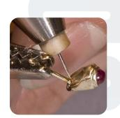
1 Hold the electrode at a 45° angle to the pin, so that the tip touches the spot where the base of the pin and the work piece meet. Now place a weld here.
