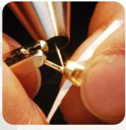
2 After the pin has been tacked from two sides, the electrode tip is placed on the edge of one of the two welds, and a new weld is placed at this point. The weld is then continued in the same manner, until a seam is formed which runs all the way around the pin. This way the welds overlap eachother, creating a very solid join.
