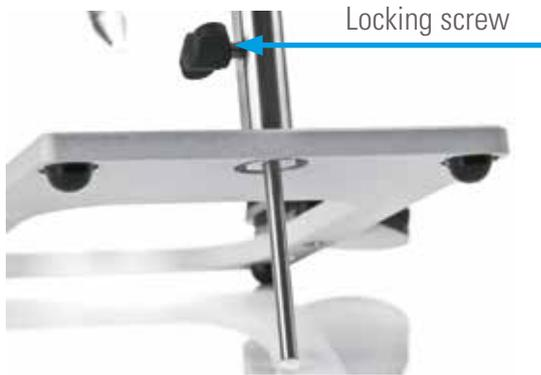
You also have the option of changing the angle of inclination for the microscope. To do so, undo the locking screw in the stand. A metal support now extends and forms an additional stand leg. Move the microscope into the desired position and tighten the screw again.
