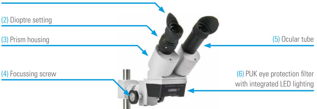
Look through the two oculars (1) and move the ocular tubes (5) inwards or outwards by moving the prism housing (3) in or out. The interocular distance is correct if the range of vision as viewed through the two oculars is complete and is united as a single complete image. The interocular distance should be individually set for each user. A spacer sleeve ensures the correct distance for focussing.
