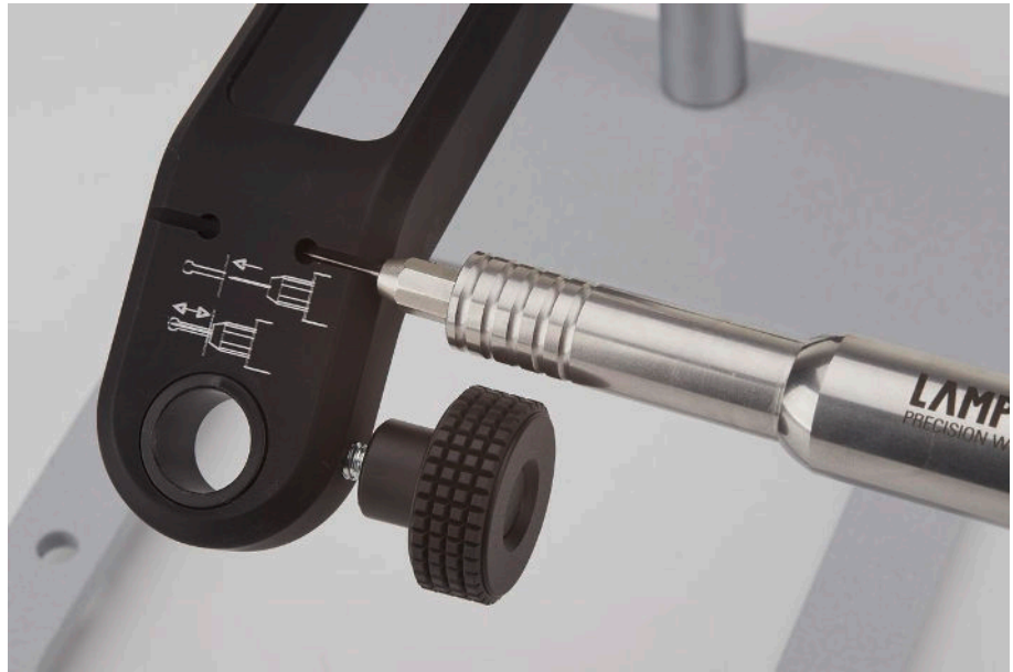
Fig. 5.2 Adjusting electrode length with handpiece holding arm
