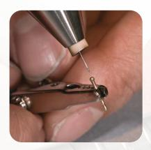
2 To increase the thickness of metal on the pin, and therefore increase the amount of metal at the joint, hold the pin with the crocodile clip, and place a weld directly on the end of the pin. During welding please place your hands on the work bench (resting position), this will make work a lot easier.
