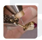
1 Hold the electrode at a 45° angle to the pin, so that the tip touches the spot where the base of the pin and the work piece meet. Now place a weld here.
