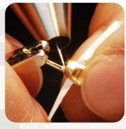
2 After the pin has been tacked from two sides, the electrode tip is placed on the edge of one of the two welds, and a new weld is placed at this point. The weld is then continued in the same manner, until a seam is formed which runs all the way around the pin. This way the welds overlap eachother, creating a very solid join.
