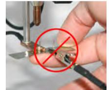
Insert the connection cable for the welding device into the corresponding outlet (13) on the PIN module and also into the corresponding outlet on the welding device (before please check and make sure that the PUK04/PUK U4 is switched off) and tighten the safety screws on the plugs by hand.
